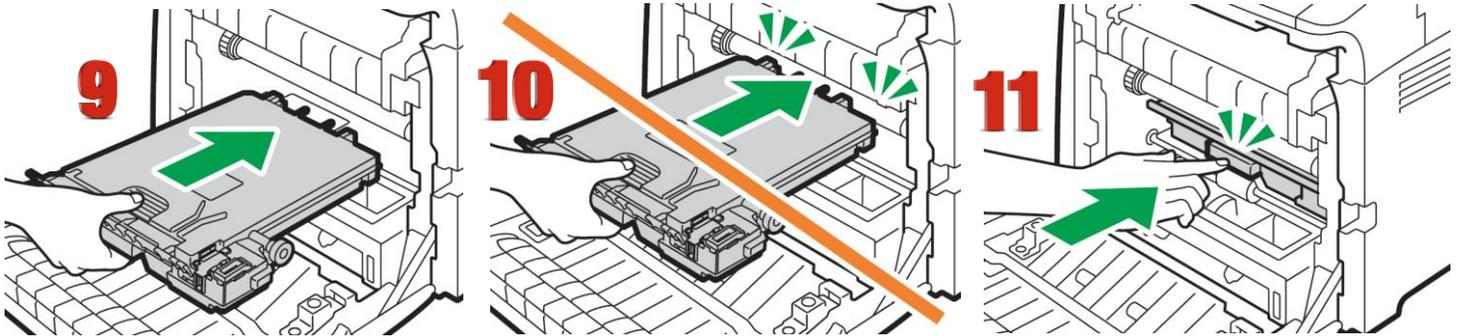
9. Holding the center of the new waste toner bottle, carefully insert it halfway into the machine body. Leave the bottle cap open.
