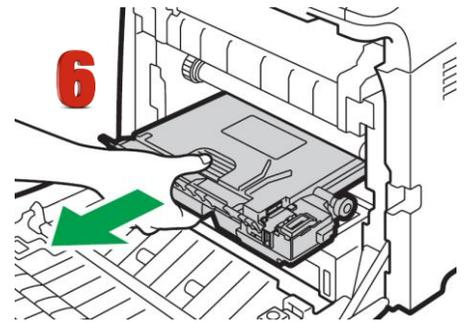
4. Holding the handle at the center of the waste toner bottle, carefully pull it partially out without tilting it.
