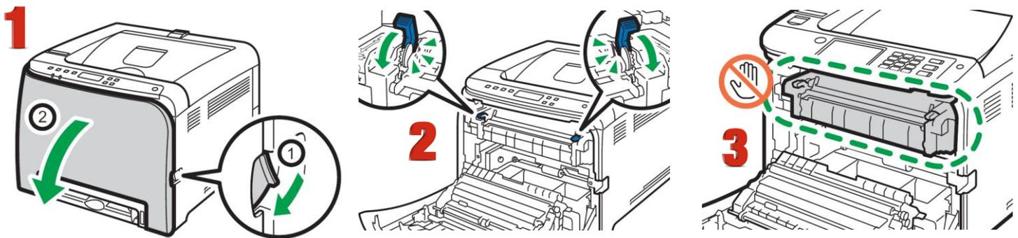
1. Pull the front cover open lever and then carefully lower the front cover.
