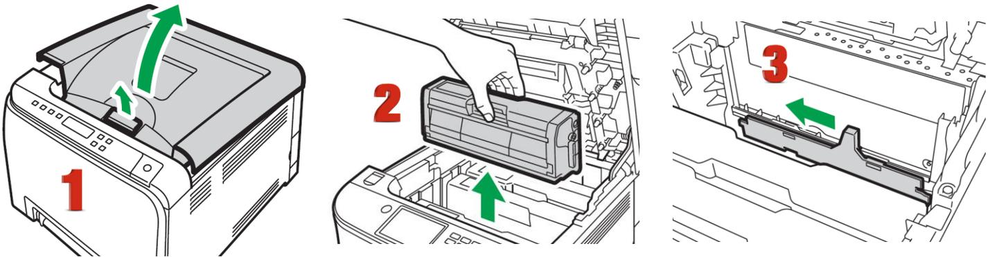
1. Pull up the lever on the top cover, and then carefully raise the top cover.
