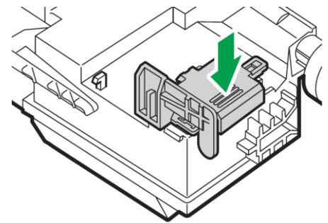
7. To prevent the waste toner bottle from coming into contact with the intermediate transfer unit (the position shown by the arrow in the illustration below), do not lift the bottle while pulling it out.
