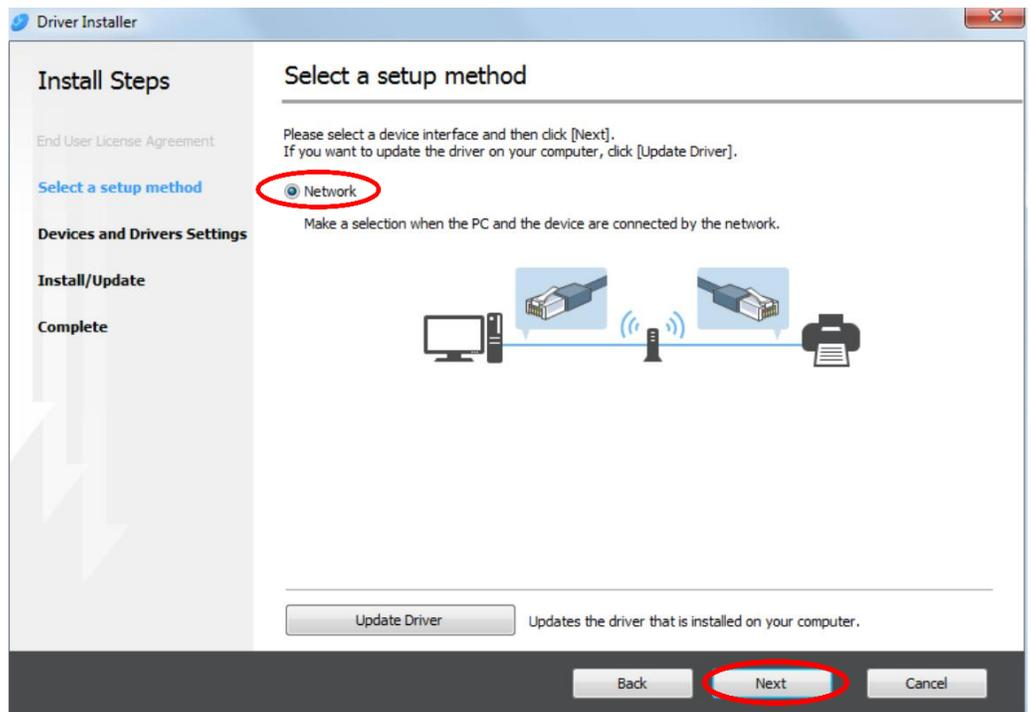
6. The software will detect the printer on your network. Click on the printer and click 'Next'. The driver will now install.
