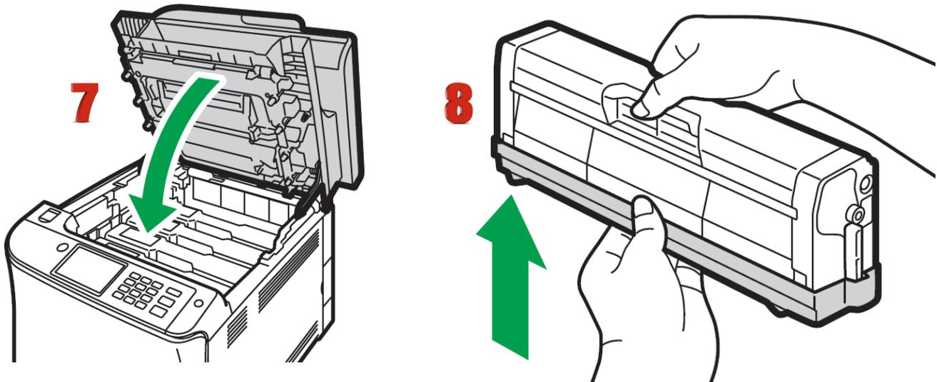
7. Using both hands, hold the center of the top cover and close the cover carefully.
