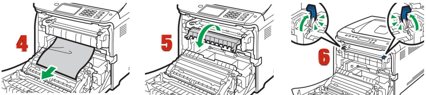
4. Pull the paper downward to remove it. Do not pull it upward.
