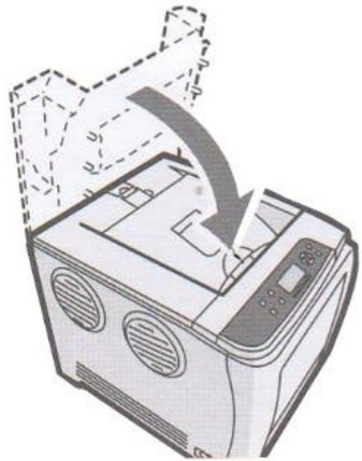
Reinstall the cartridges in the desired configuration (in the above representation, white or black can go into the first slot) and close the lid. Use white for transfer printing and black for normal CMYK printing.
