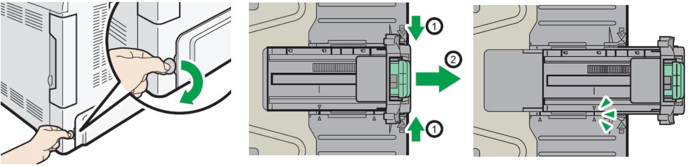
When loading paper longer than 11” into tray 1, remove the lower rear cover using a coin. Squeeze the rear extender and push outward to accommodate lengths up to 14” long. Do not extend this tray when loading A4 or letter size paper. Otherwise, a paper jam may occur.
