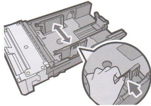
Squeeze the clips on the paper guides and slide them to match paper size. Do not move the paper guides forcefully. Doing so may damage the tray.
