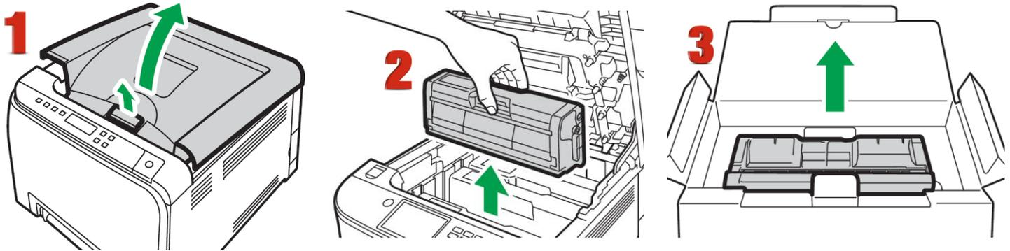
1. Pull up the lever on the top cover, and then carefully raise the top cover.
