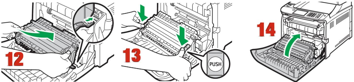
12. Place the transfer unit on the front cover. Slide the transfer unit along the guide rails into the machine.
