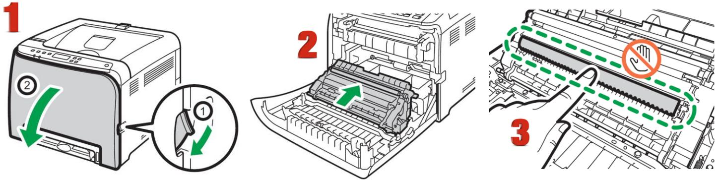
1. Turn off the power and unplug the power cord. Pull the front cover open lever and then carefully lower the front cover. Be sure to set the registration roller in the position shown by the arrow in the illustration below. Do not touch the transfer roller.
