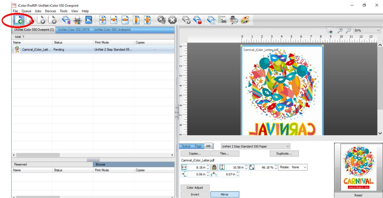
10) There are preloaded images that can be used to print a test page. Click **Devices >> Print Test Page** to see the choices. It is suggested that you print a test page upon completion of the setup to confirm the printer has been properly installed. Use [Shift] and [Ctrl] to click multiple pages, and then click OK. More about the uses of each page can be found in the Help Topics file within the ProRIP program.
