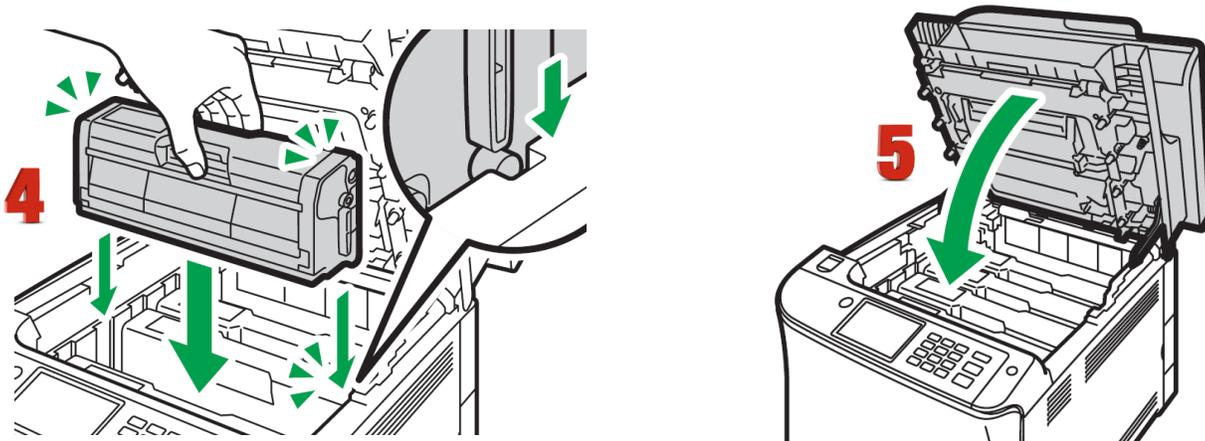
4. Carefully insert the print cartridge removed in Step 2 vertically.
