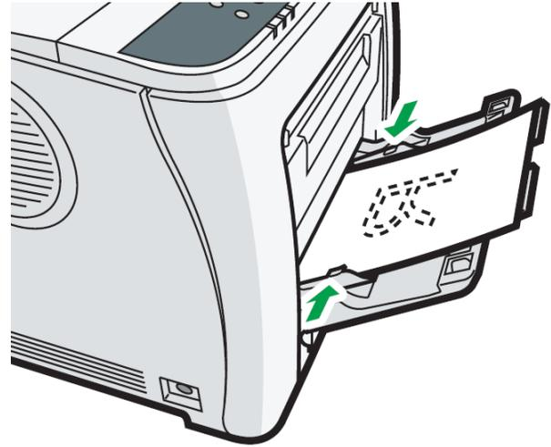
Load the paper print side face down and adjust the guides as necessary.
